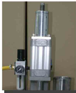
High power cylinder with adjustable stopper.
